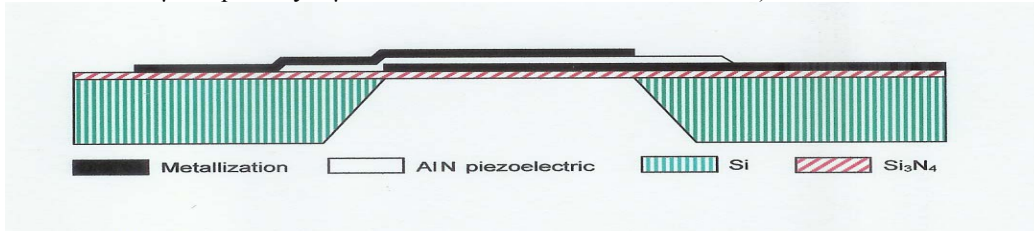
Figure 6. Basic FBAR construction (cross-section side view, not to scale).
