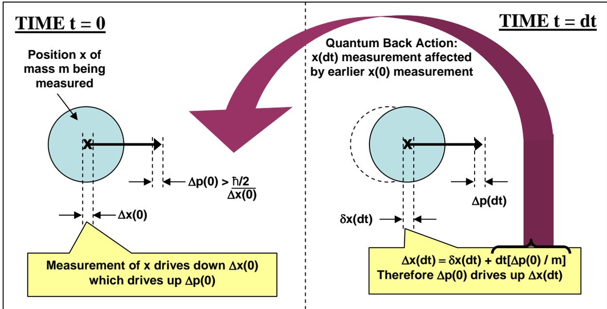
FIGURE 1. An example of how quantum back action is the mechanism for creating the standard quantum limit
