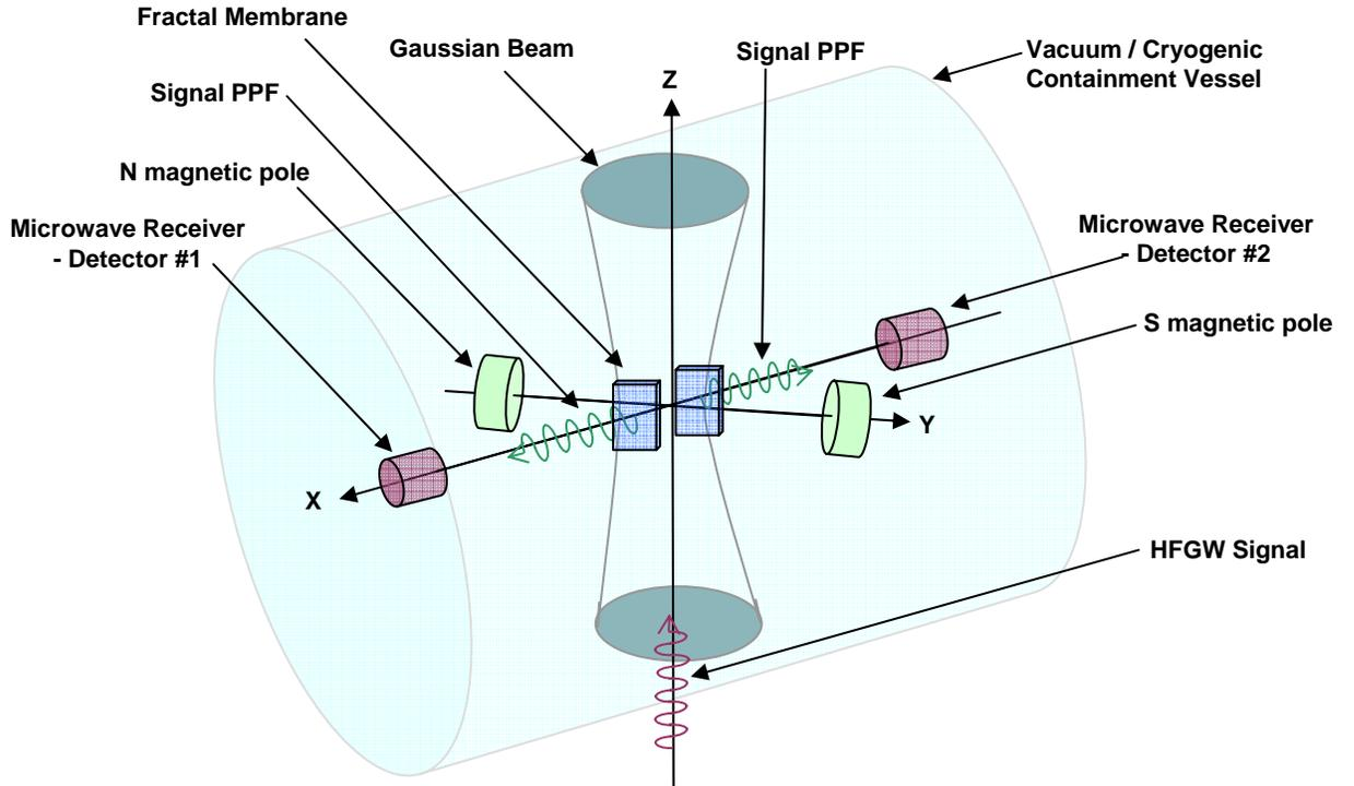
FIGURE 2. The configuration of the Li-Baker Energy Resonance Detection System.
