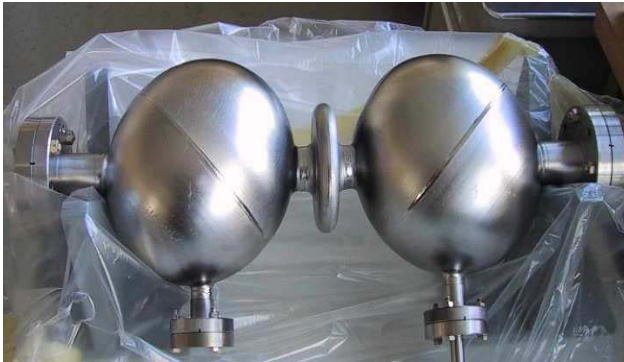
Figure 3.6.2b. INFN Genoa HFGW Detector
